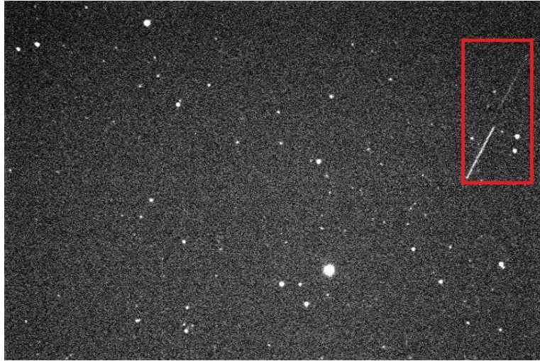
Figure 2: AROAC-T08 acquisition on 24.07.2020: Low conjunction probability between COSMOS 2543 and COSMOS 2535 satellites. The stars appear as stable points while space objects as tracked (© Romanian Academy Cluj-Napoca Branch, Astronomical Observatory Cluj-AROAC, 2020)
