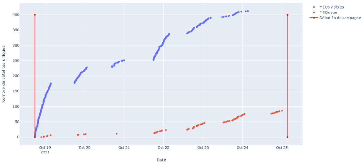
Figure 9: Number of MEO objects that can be theoretically observed by the MEO strategy (in blue) and number of objects detected during the operational campaign as a function of time
