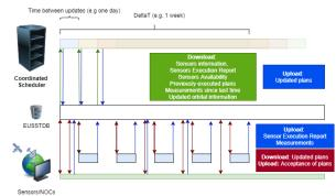
Figure 6: Schematic timeline with nominal interactions Sensors-OC-EUSST DB-Coordinated Scheduler
