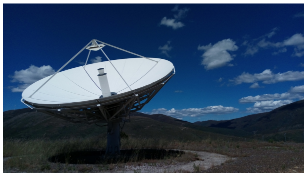
Fig. 1. ATLAS the 5.56 GHz monostatic radar tracking sensor located at PASO.
