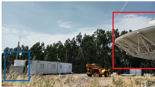
Fig. 3. In this picture taken at PASO it is visible the telescope dome during its installation (in blue), and the ATLAS radar antenna dish (in red). The two sensors are only about 34 m apart.
